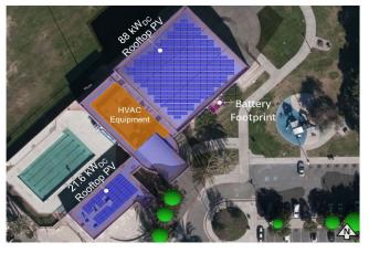
Snapshot of photovoltaic (solar) and battery storage system layout recommended for a SoCalREN public agency facility
